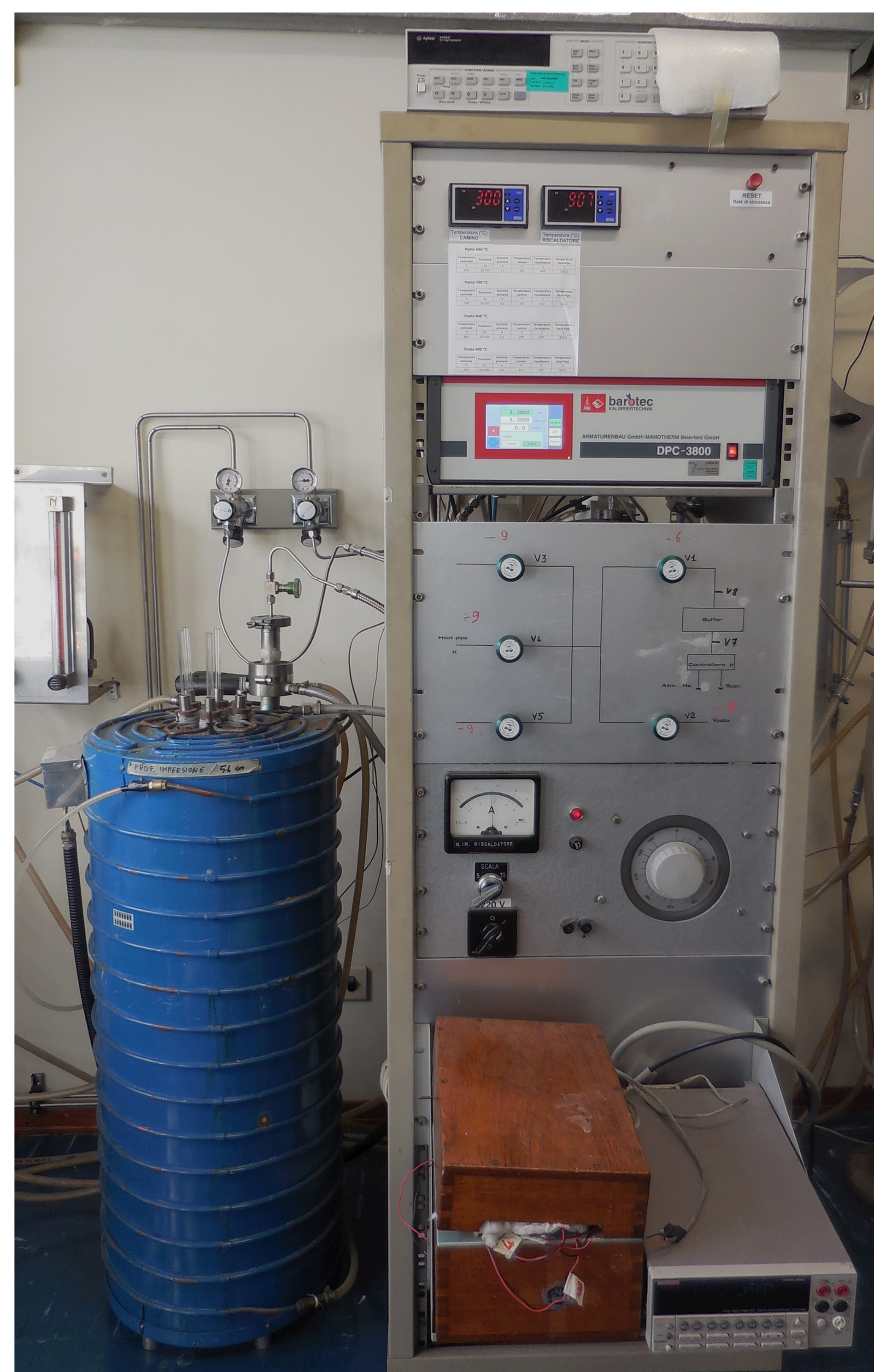
A sodium gas controlled heat pipes for temperatures up to 960 °C
