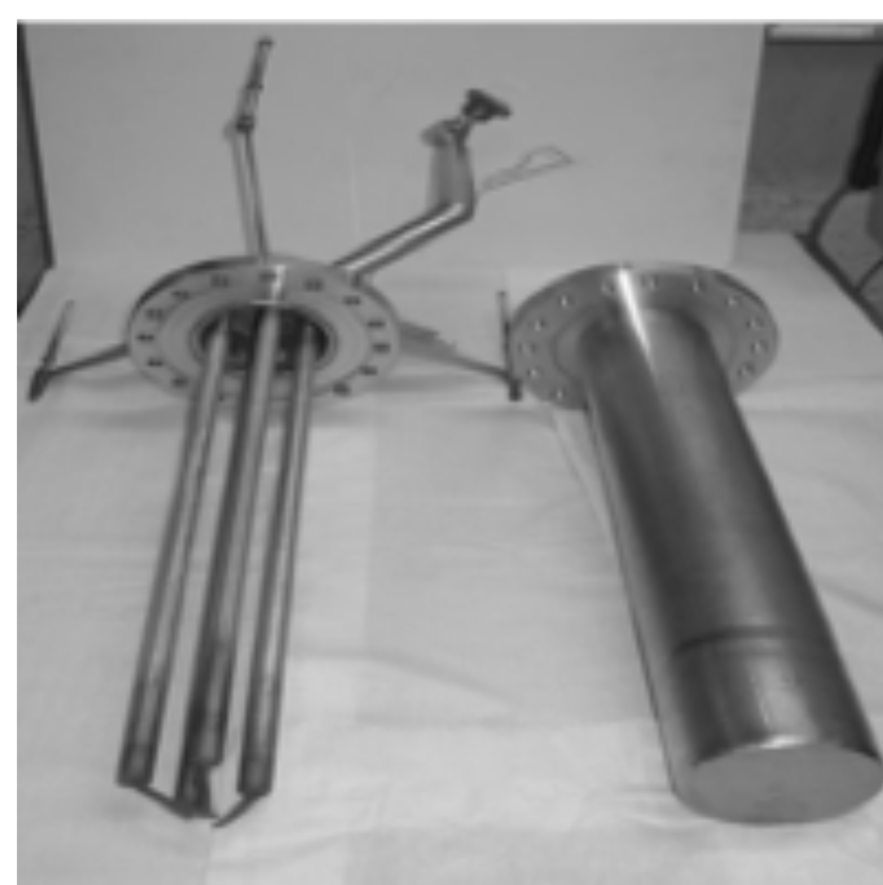
Typical design of a modern gas controlled heat pipe for lower temperatures (80 °C to 400 °C).
