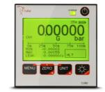
HALT Froze the display at the actual measuring value DISPLAY MODE Sets the active channel on the display LOG SAMPL TIME Sets the sampling tome of the datalogger (up to 8 log in csv format downloadable by RS-232 port) LOG TIME Period in time of the log LOG SLOT Software slot of the log recording (csv file) LOG Sets the LOG on and off (if the log is on a blinking icons is shown on the screen while recording)
